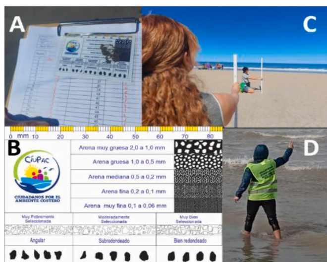
Fig. 4. Monthly monitoring activities. A. Sediment characterization; B. Beach profile measurement; C. Reference chart for visual sediment analysis; D. Longshore current observations.
